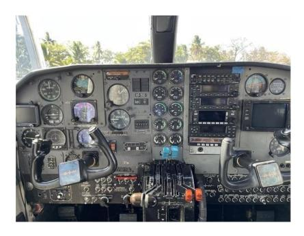
Audio panel, radios and transponder are Garmin and its ADSB equipped. KLN90 GPS.
